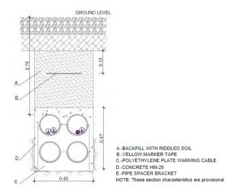
Figure 5-42 Example of buried PVC ducts
