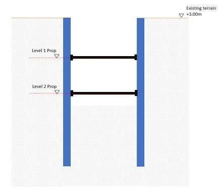
Figure 5-177 Phase 4 – excavation to bottom slab level
