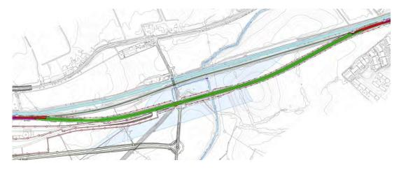
Figure 5-347 Phase 5 new double track diversion (green)
