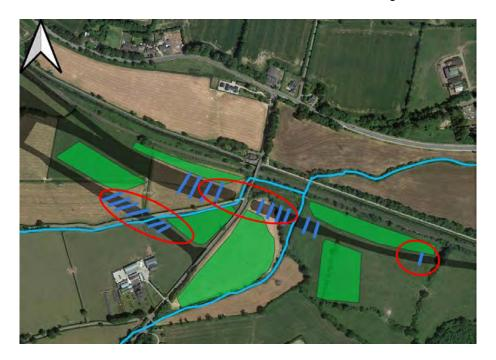
Figure 5-376 Indicative location of flood relief culverts (in red)
