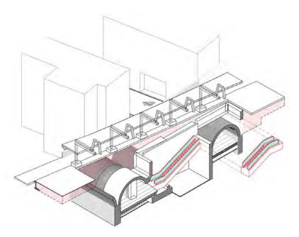
Figure 5-111 3D view of step 10 - installation of escalators
