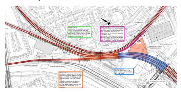
Figure 5-189 Spencer Dock proposed walls and protection slabs with the final track alignment
