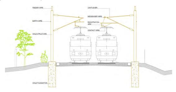
Figure 5-80 Standard OHLE structure
