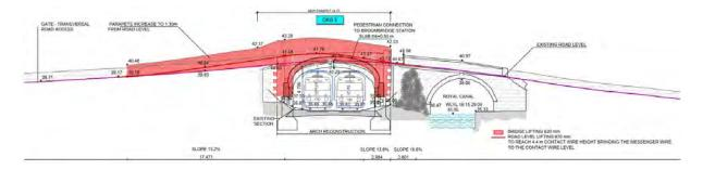
Figure 5-230 Elevation of OBG5 deck reconstruction
