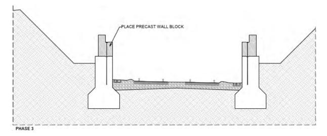
Figure 5-49 Placement of the precast concrete wall blocks
