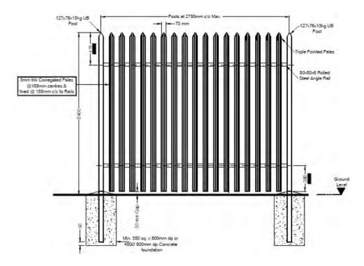
Figure 5-87 Security purpose (SP) fencing
