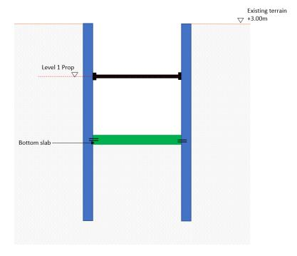
Figure 5-179 Phase 6 – removal of lower prop
