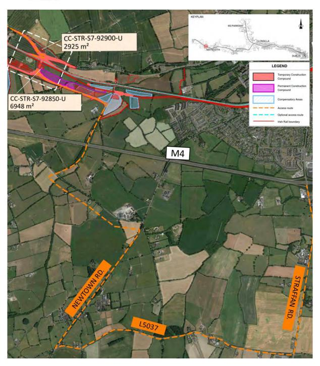
Figure 5-372 OBG23A Construction compounds and haulage routes
