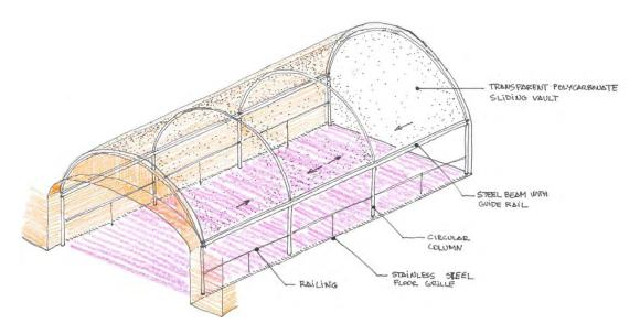
Figure 5-115 Sketch of transparent polycarbonate umbrella inside vault
