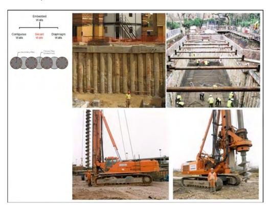
Figure 5-34 Typical plant required for secant piling
