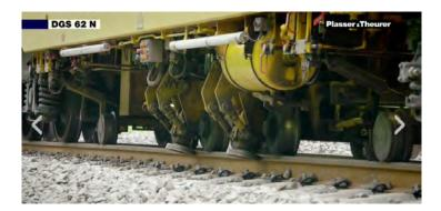
Figure 5-27 Extension of second ballast layer, tamping and dynamic stabilisation
