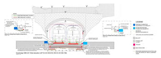
Figure 5-221 Section showing proposed L-form retaining wall at OBD221
