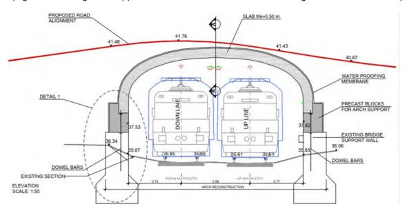
Figure 5-45 Structural elevation of OBG5
