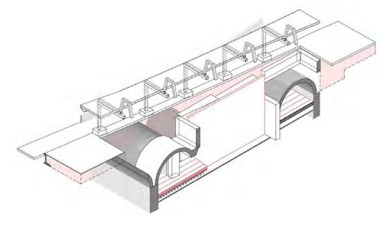
Figure 5-110 3D view of step 9 - escalator shaft construction
