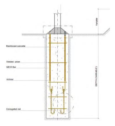
Figure 5-78 Standard OHLE foundation
