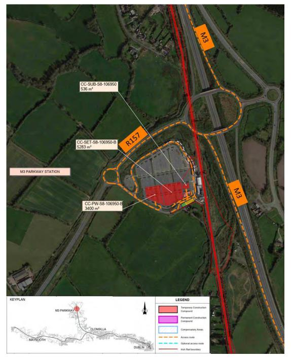
Figure 5-295 M3 Parkway permanent way construction compound and haulage route
