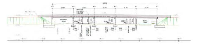
Figure 5-369 Elevation of proposed solution for OBG23A
