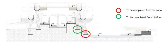
Figure 5-241 Section through Ashtown pedestrian bridge showing foundations
