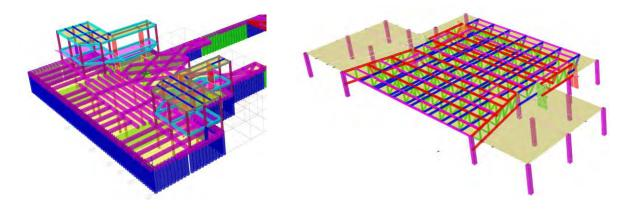
Figure 5-152 Numerical structural model of reinforced concrete structure (left) and steel roof structure (right)
