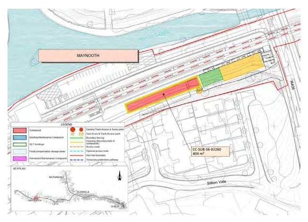
Figure 5-333 Maynooth substation compound
