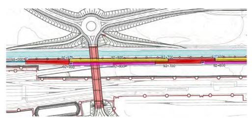
Figure 5-352 Phase 10 crossover & turnout installation (red)
