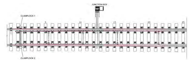
Figure 5-70 Typical heater strips & clamplocks lay-out
