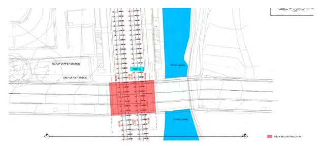
Figure 5-306 Plan of OBG14 deck reconstruction
