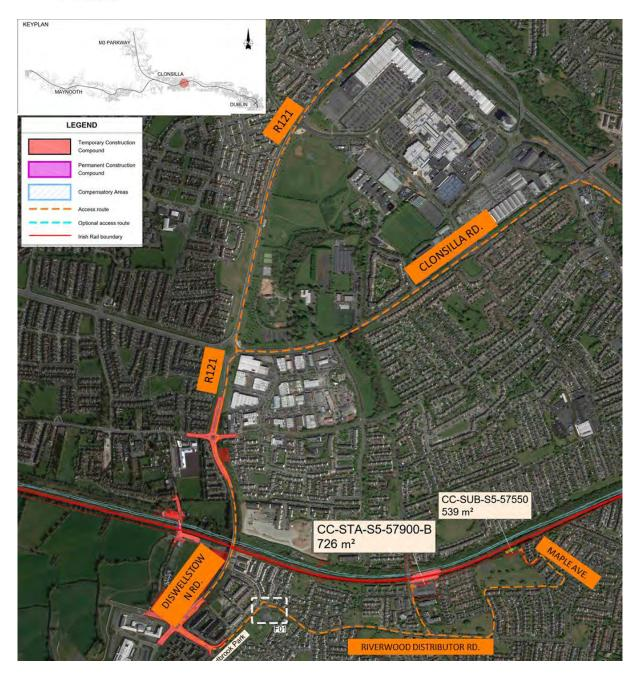
Figure 5-270 Coolmine Station compound and haulage route
