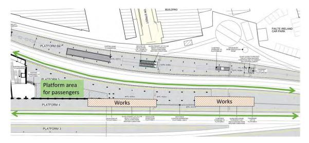
Figure 5-98 Simultaneous construction and operation on platform 5
