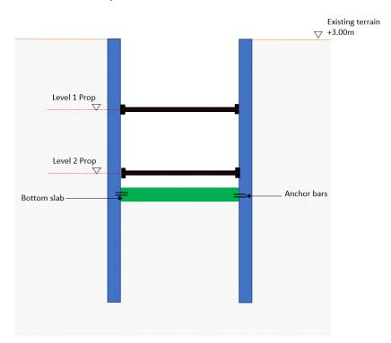
Figure 5-178 Phase 5 – construction of bottom slab
