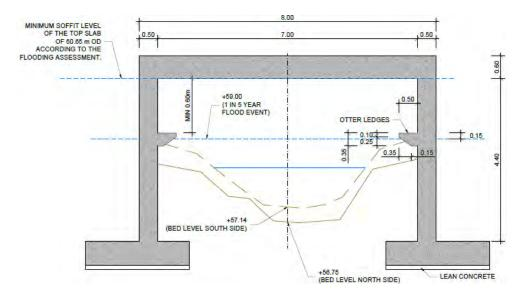
Figure 5-363 Cross section of UBG22B
