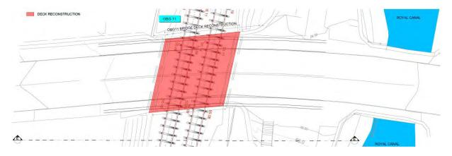
Figure 5-259 Plan of OBG11 deck reconstruction
