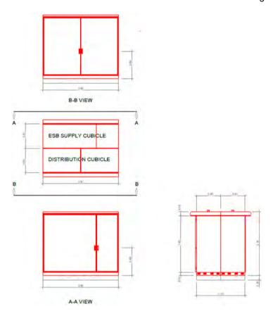
Figure 5-68 Double sided DNO/distribution cubicle board
