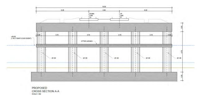
Figure 5-361 Section A-A - proposed pier design
