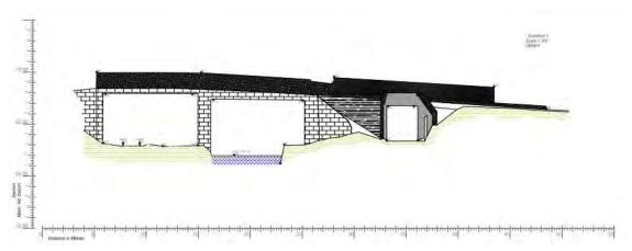
Figure 5-388 Plan (above) and elevation (below) of OBG24 (bridge and underpass for Royal Canal greenway)
