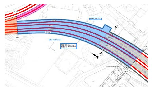
Figure 5-190 Spencer Dock proposed walls and protection slabs - Structure A
