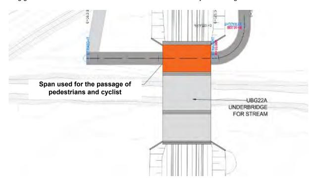
Figure 5-359 Location and plan view of UBG22A
