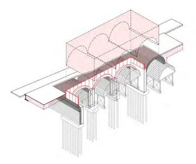
Figure 5-105 3D view of step 5 – excavation down to falsework level
