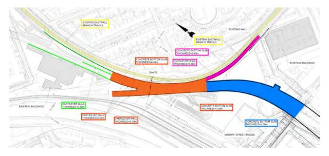
Figure 5-203 Phase 4 - construction of cantilever walls and bottom slabs
