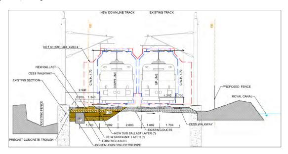
Figure 5-342 Section of new track (Down track) between the existing track and the depot.
