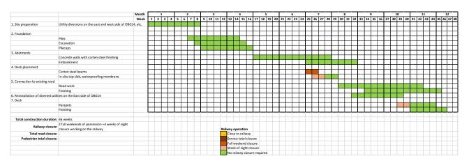
Figure 5-310 Construction duration of east and west footbridges (duration indicated is for one footbridge)
