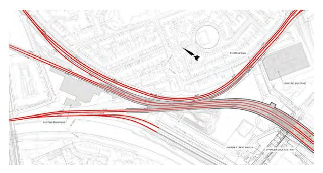
Figure 5-204 Phase 6 - placement of new tracks
