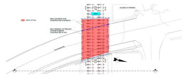
Figure 5-252 Plan of OBG9 deck lifting
