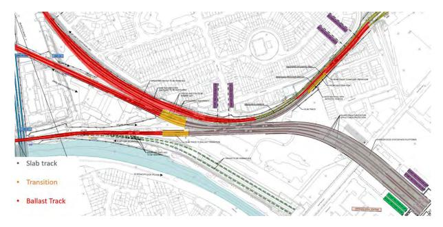
Figure 5-186 Ballast and slab track solutions in Spencer Dock area
