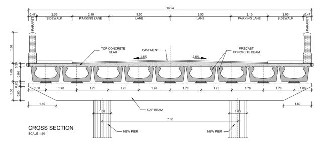
Figure 5-171 OBD228 - reconstructed cross section
