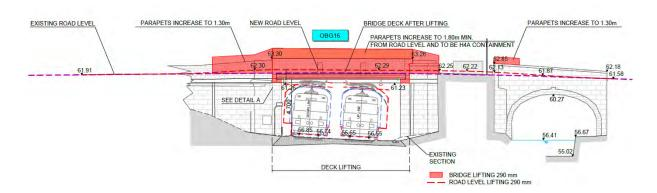
Figure 5-318 Elevation of OBG16 deck lifting
