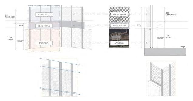
Figure 5-89 Design intent for parapet heightening on bridges
