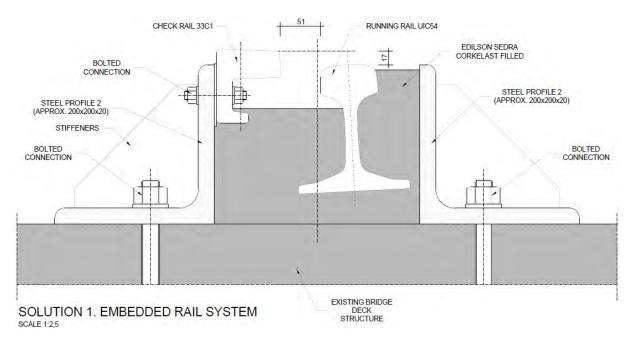
Figure 5-216 Solution 1 - Proposed embedded rail system.
