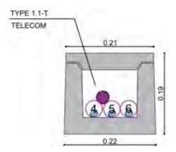
Figure 5-41 Example of precast concrete trough
