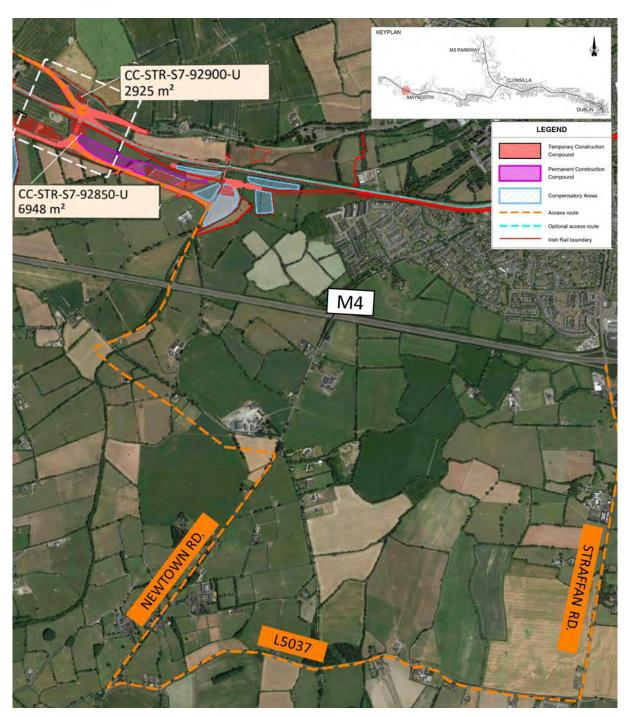
Figure 5-375 OBG23A construction compounds and haulage routes
