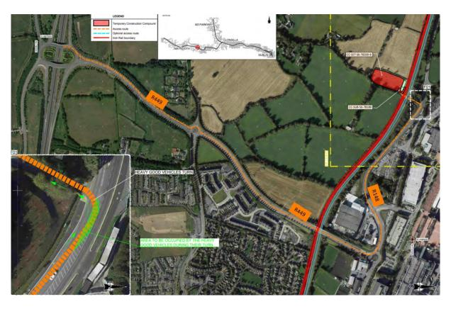
Figure 5-326 Blakestown substation compound and haulage route
