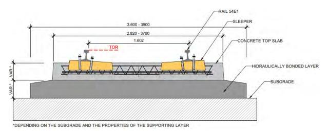
Figure 5-28 Schematic of concrete slab track (the concrete embedded sleeper solution shown is an example of the solution initially proposed in the report pending approval)
