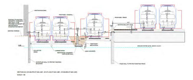
Figure 5-199 Structure D - cross section
