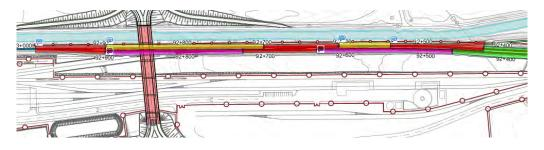
Figure 5-350 Phase 8 track realignment (yellow)
