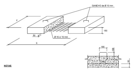
Figure 5-9 Precast slab with embedded hooks.
