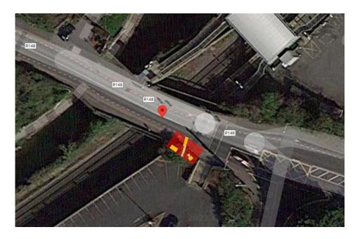
Figure 5-320 Plan of proposed temporary material storage area at OBG16
