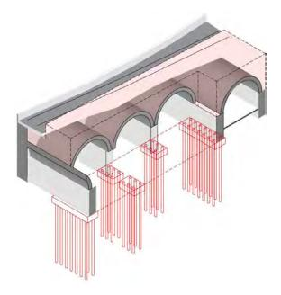
Figure 5-99 3D view of step 1 – foundation construction
