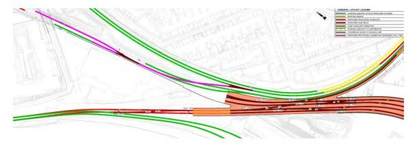
Figure 5-210 Constructed Pway before the provisional connection removal
