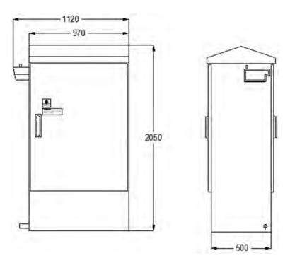
Figure 5-66 Points heating control cubicle indicative dimensions
