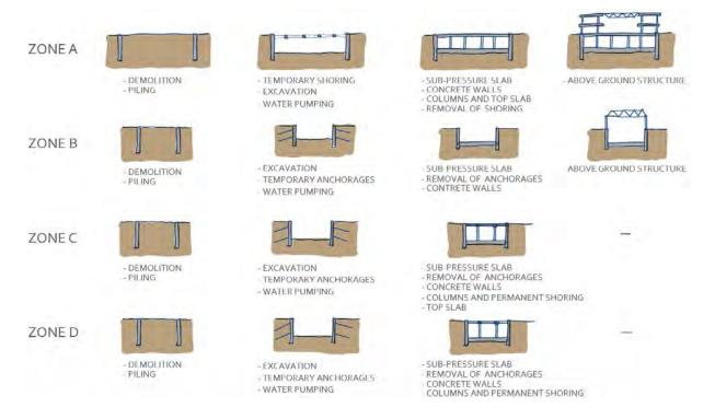
Figure 5-163 Schematic of Spencer Dock Station construction phases
