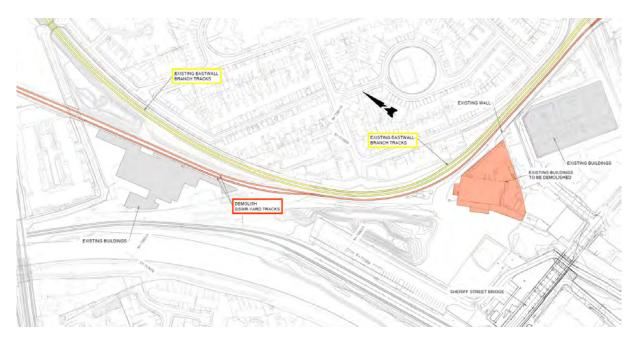
Figure 5-200 Phase 2 - demolition of existing tracks and buildings
