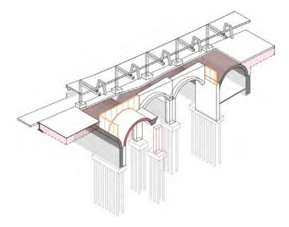
Figure 5-108 3D view of step 7 – arched slab construction
