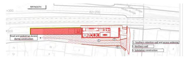
Figure 5-334 Maynooth substation road and pedestrian access
