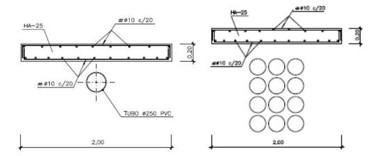
Figure 5-8 Slab based utilities protection.
