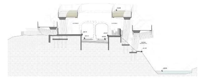
Figure 5-269 Section through Coolmine pedestrian bridge showing foundations
