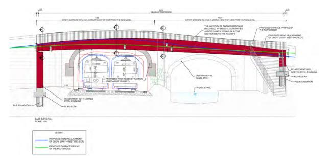
Figure 5-308 East elevation of proposed east footbridge structure
