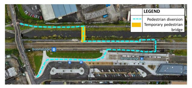
Figure 5-233 Pedestrian diversion via temporary ramp at OBG5
