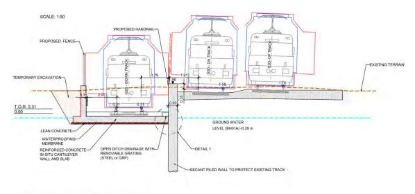
SECTION B2-B2 (CH 25+210 AT S2B LINE - CH 28+280 AT S2D LINE)
