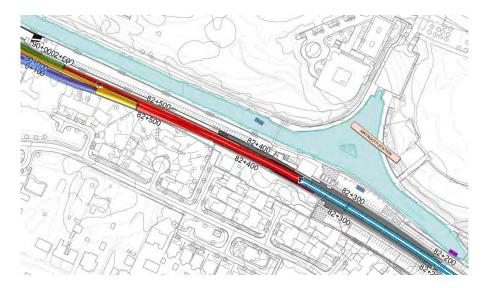
Figure 5-354 Maynooth station track realignment & crossover replacement (red)
