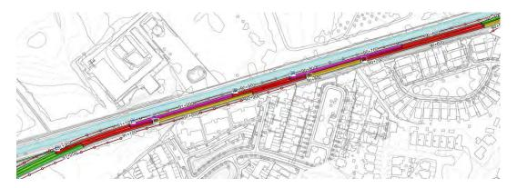
Figure 5-349 Phase 7 track realignment (yellow)
