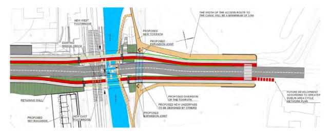
Figure 5-307 Plan of proposed footbridges to east and west of OBG14
