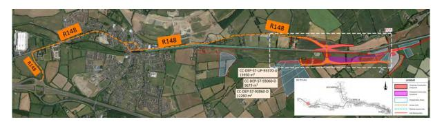
Figure 5-386 Depot siding construction compound and haulage route
