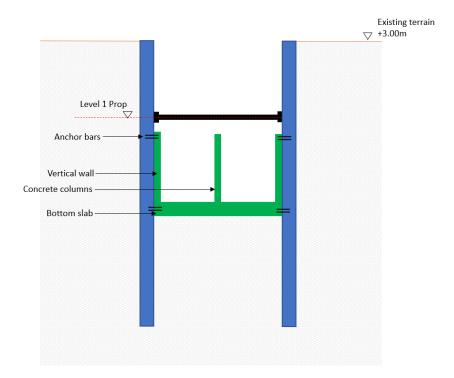
Figure 5-180 Phase 7 – construction of tank walls and columns
