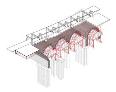
Figure 5-103 3D view of step 3 - erection of falsework
