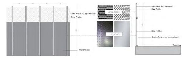
Figure 5-91 Design intent for parapet heightening on footbridges
