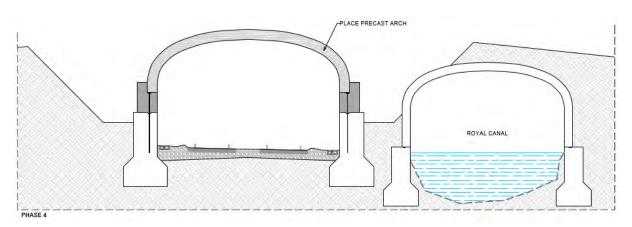
Figure 5-50 Placement of the precast concrete arch deck
