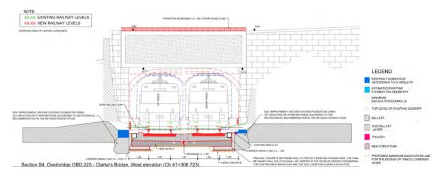
Figure 5-218 Section showing proposed L-form retaining walls at OBD225
