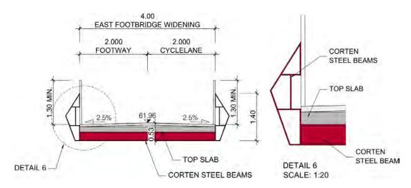
Figure 5-309 Cross section of footbridge deck (indicative cross section outside of railway area)
