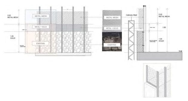
Figure 5-93 Design intent for parapet heightening on walls
