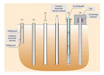
Figure 5-35 Execution process for micropiles
