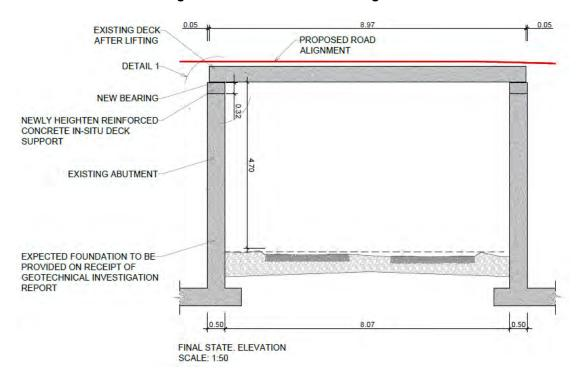
Figure 5-58 Elevation of OBG9 following deck lifting intervention
