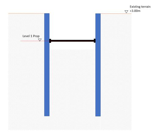
Figure 5-176 Phase 3 – excavation to top slab level
