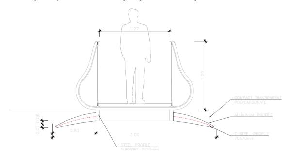
Figure 5-92 Proposed parapet solution at OBG12 Clonsilla station footbridge
