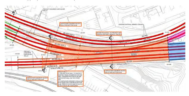
Figure 5-195 Spencer Dock proposed walls and protection slabs - Structure C
