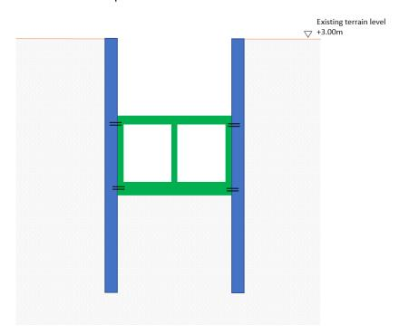
Figure 5-182 Phase 9 – removal of remaining prop
