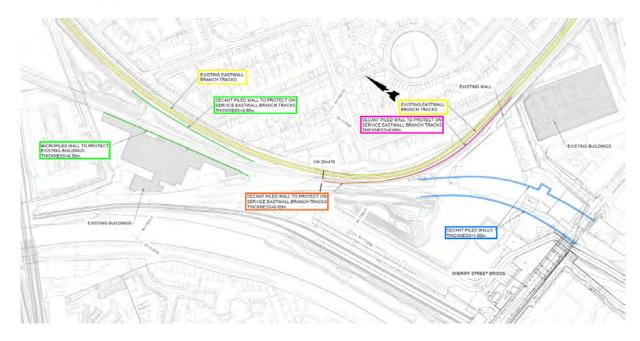
Figure 5-201 Phase 3 - construction of piled walls
