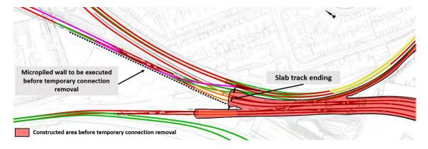
Figure 5-209 Area to be constructed before the provisional connection removal
