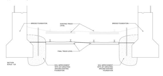
Figure 5-60 Soil improvement around existing foundation before excavation
