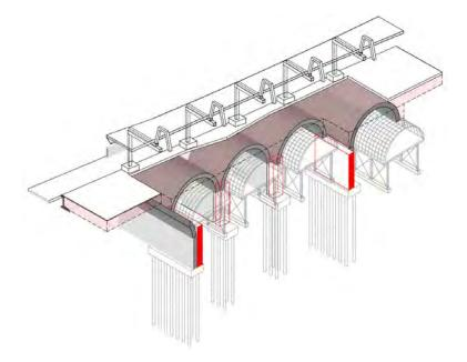
Figure 5-104 3D view of step 4 – construction of shaft columns
