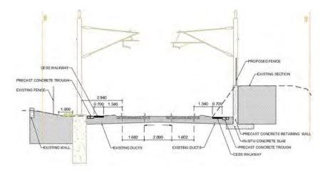
Figure 5-33 Example of cantilever retaining wall solution
