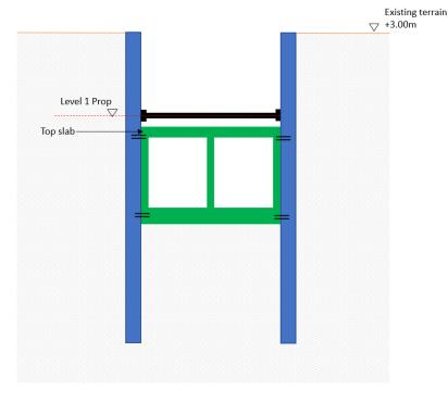
Figure 5-181 Phase 8 – construction of top slab
