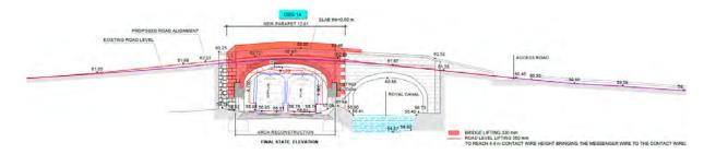
Figure 5-305 Elevation of OBG14 deck reconstruction
